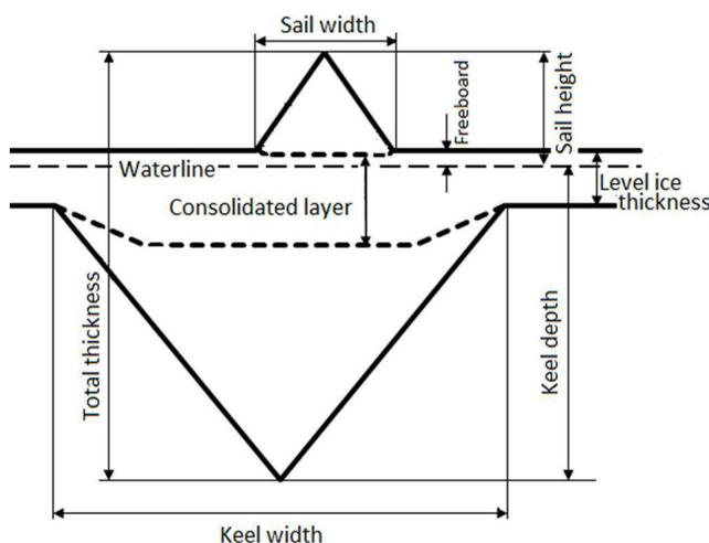
Fig. 1 Diagram of an ice ridge cross section. “Freeboard” is the elevation of the ice in the ridge above the waterline.
