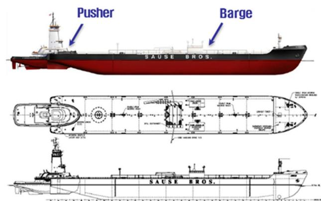
Fig. 1 General arrangement of a pusher–barge system
