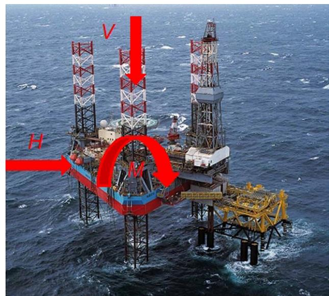
Fig. 1 A typical jack-up platform and the loading conditions
