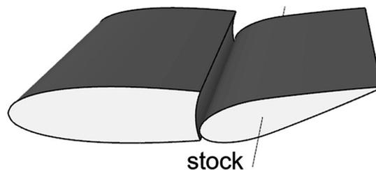
Fig. 1 Conventional submarine stern control surface
