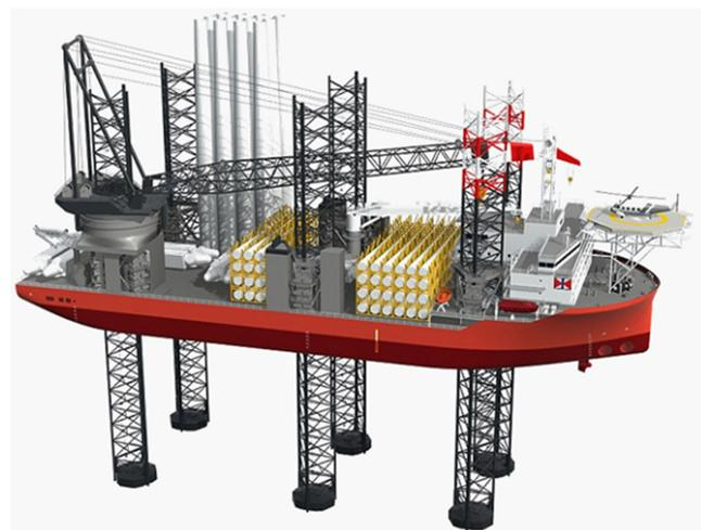
Fig. 1 Wind turbine installation vessel
