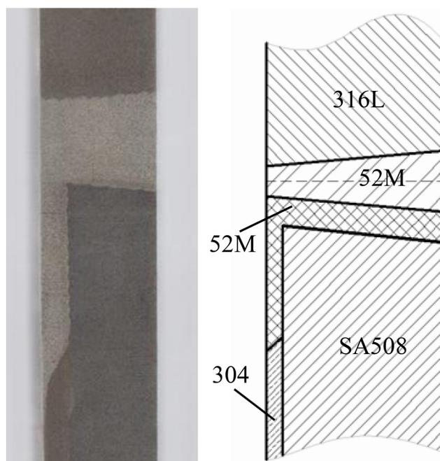
Fig. 1 Schematic diagram of the material component of a dissimilar welded joint in a pressure vessel
