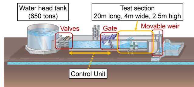
Fig. 1 Large-scale tsunami physical simulator
