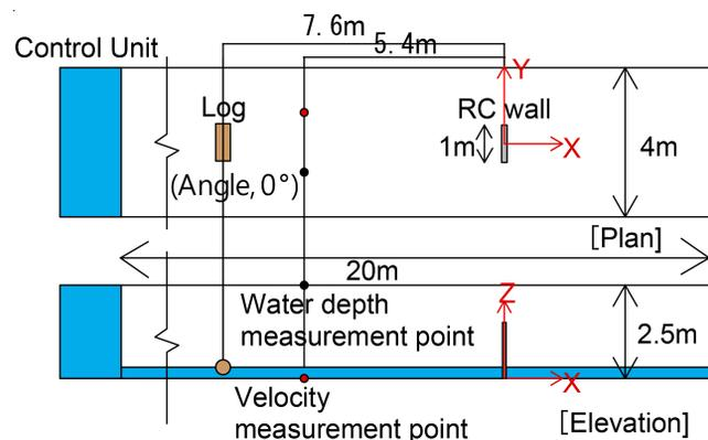
Fig. 2 Experimental setup and coordinate system
