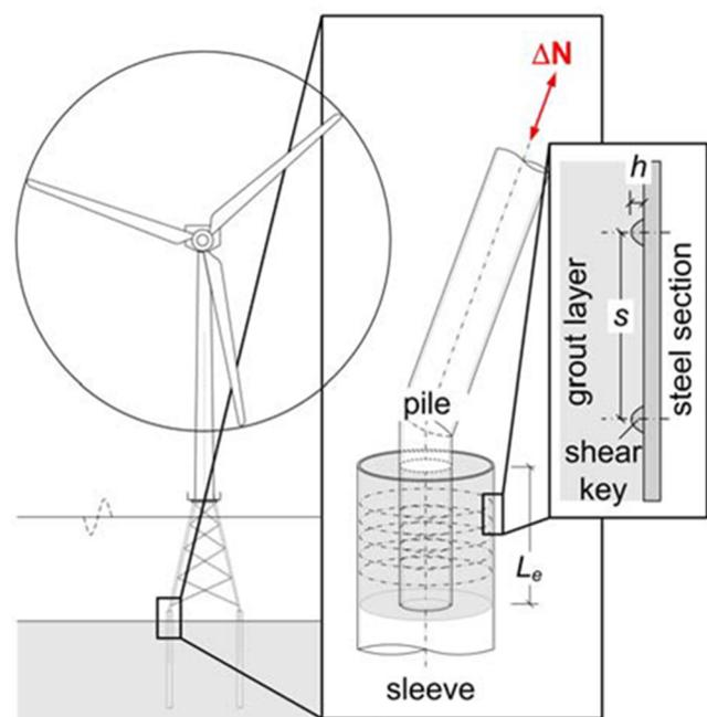
Fig. 1 OWT with jacket substructure and detail of the grouted joint (Schaumann, Bechtel and Lochte-Holtgreven, 2010)
