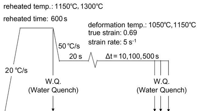
Fig. 1 Test conditions of hot processing simulator
