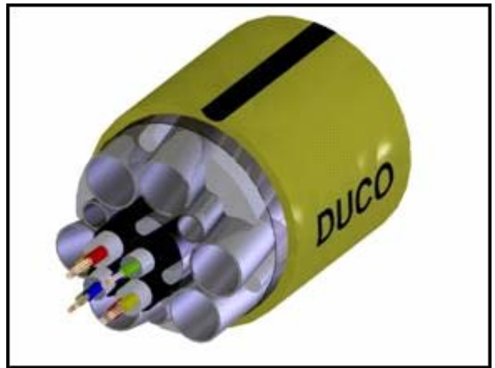
Figure 1 – Typical Steel Tube Umbilical
