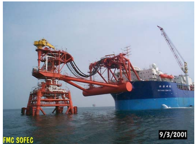
Fig. 1 Tower-yoke mooring system for CNOOC QHD 32-6 FPSO
