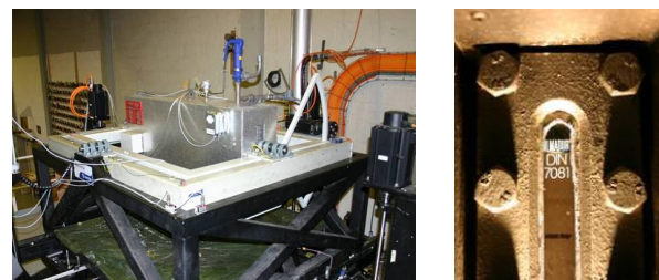
Fig. 1 Left: General view of experimental set-up; right, small window to check boiling level
